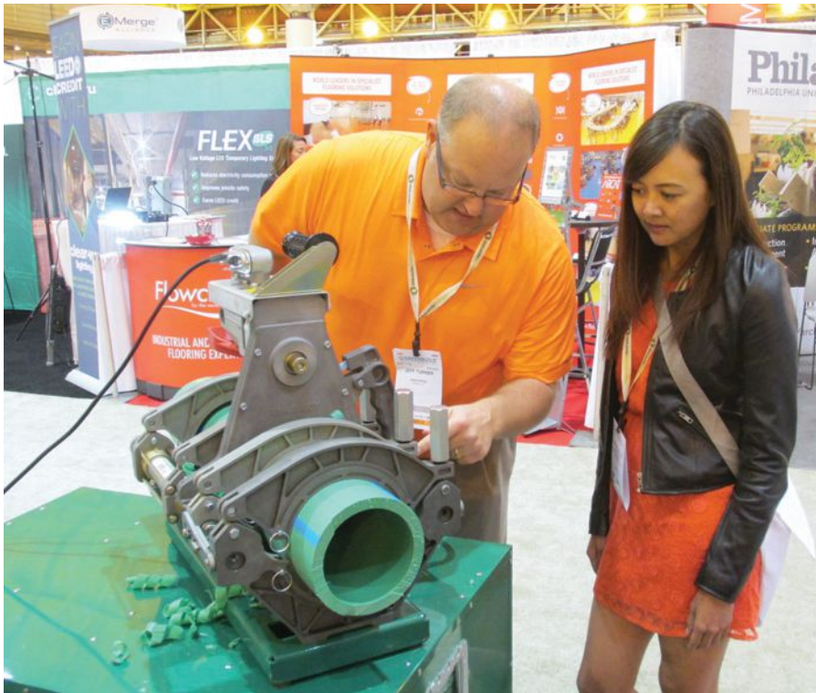
MEP Engineer Shawn Wilson of Interface Engineering in San Francisco watches Jeff Turner of McElroy Manufacturing butt-weld polypropylene pipe during a product demonstration in Aquatherm's booth Oct. 23 at Greenbuild in New Orleans. The tool, McElroy's Acrobat 160, allows installers to work in tight spaces.
